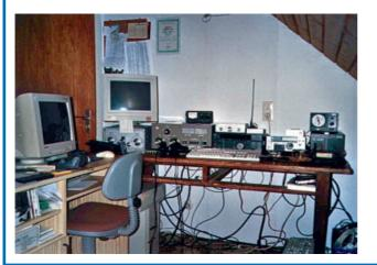
I erect a vertical for 40-160 in neighbours' farmland... (only during winter contests). In the shack I use a TS850 with Alpha78 and IC735 + SB1000 as 2nd station. Due to the limited antenna situation and interference problems I often operate from remote locations or in M/S-activities.
