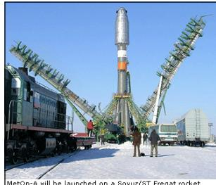
MetOp-A will be launched on a Soyuz-ST Fregat rocket from the Baikonur Cosmodrome in Kazakhstan on 17 July 2006. The launcher consists of three stages, all of which use liquid oxygen and kerosene as fuel.
